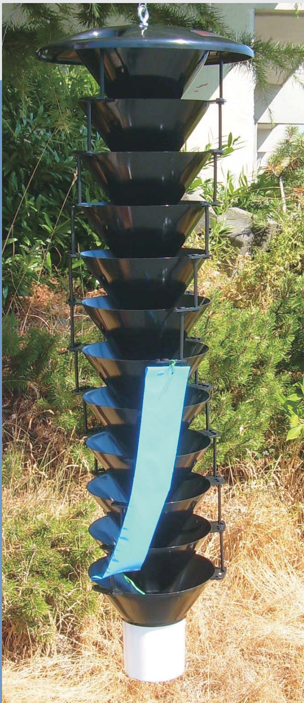
Proper placement of a full size UHR on a MultiFunnel Trap
