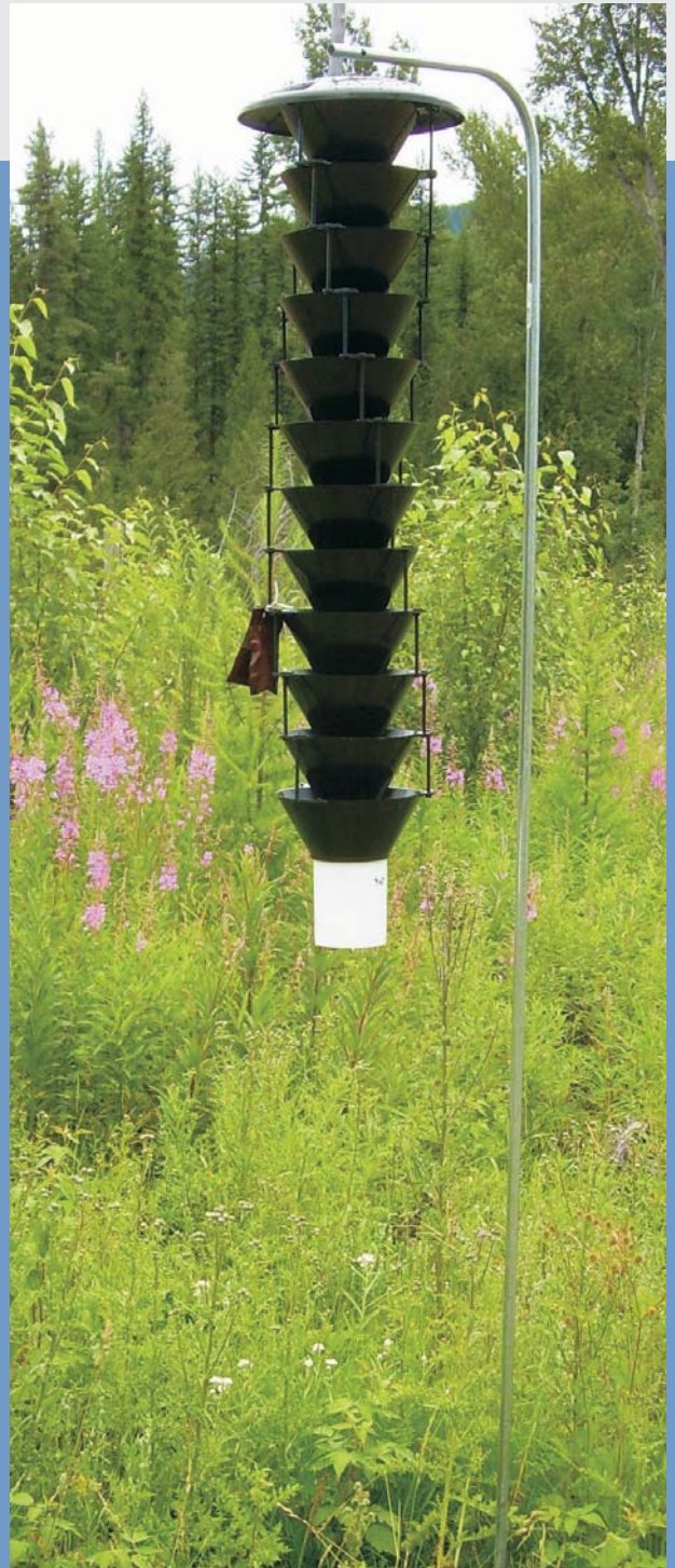
A light weight trap stand made from 1/2" diameter electrical conduit devised by Dr. Art Stock (BC Ministry of Forests) and used in place of the original heavy steel rebar.
